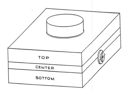
Before final assembly, the switch box should be painted a bright color contrasting with the color of the plastic cap. Lead-free paints should be used.
