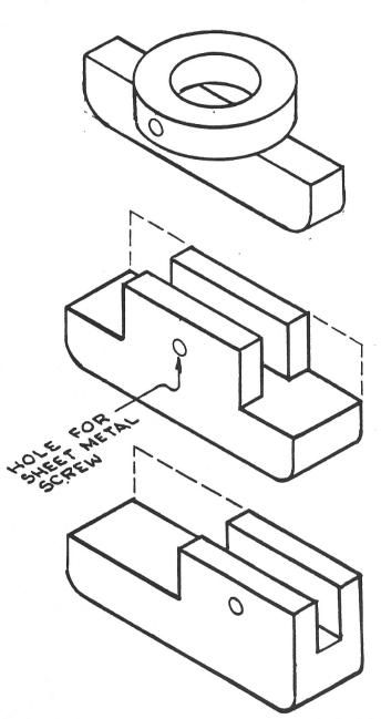
The circular plywood piece of this handle extension is to have the center hole cut using an adjustable circle cutter (Stanley Tools) to fit the knob. The outer circle is sawn on a jigsaw and sanded to an outside diameter slightly smaller than the recess in the toy where the knob is. The crossbar is attached to the ring with glue.
